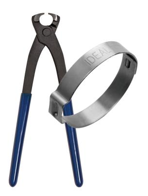
**Pinch Clamps** are designed to fit most popular polyethylene and polybutylene water service lines, and are perfect for sprinkler systems, irrigation systems and most other low-pressure applications. To determine proper pinch/crimp clamp size, measure actual outside diameter (O.D.) of the hose on the fitting. Select the nominal size clamp nearest to that size, but always larger than the O.D. of the hose on the fitting.
